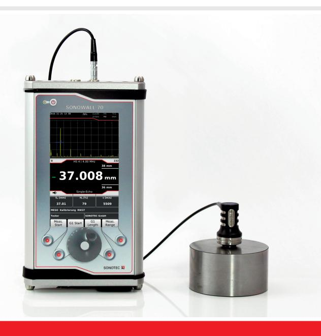
**ULTRASONIC A-SCAN/B-SCAN THICKNESS GAUGE**
