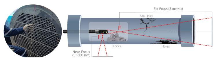
Long-length probe (5 m/7 m/10 m) tip's sophisticated DOF and FOV Optical design dedicated to tube inspection needs.
