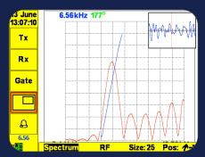
Spectrum view with phase, and RF waveform inset window.
