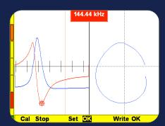
Air calibration for Resonance mode probes.
