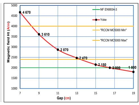
\*The general performance figures provided are indicative as they are specific to each system and may therefore vary slightly. The measurements were taken on a ISO9934-3 C22 metal plate.
