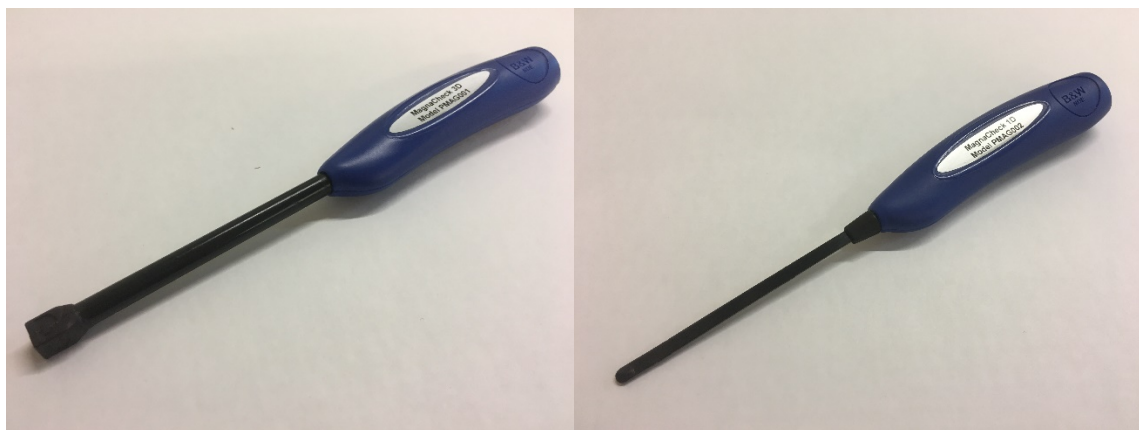
Figure 1 - 3D Magnetic field strength probe (left), 1D Magnetic field strength probe (right).
