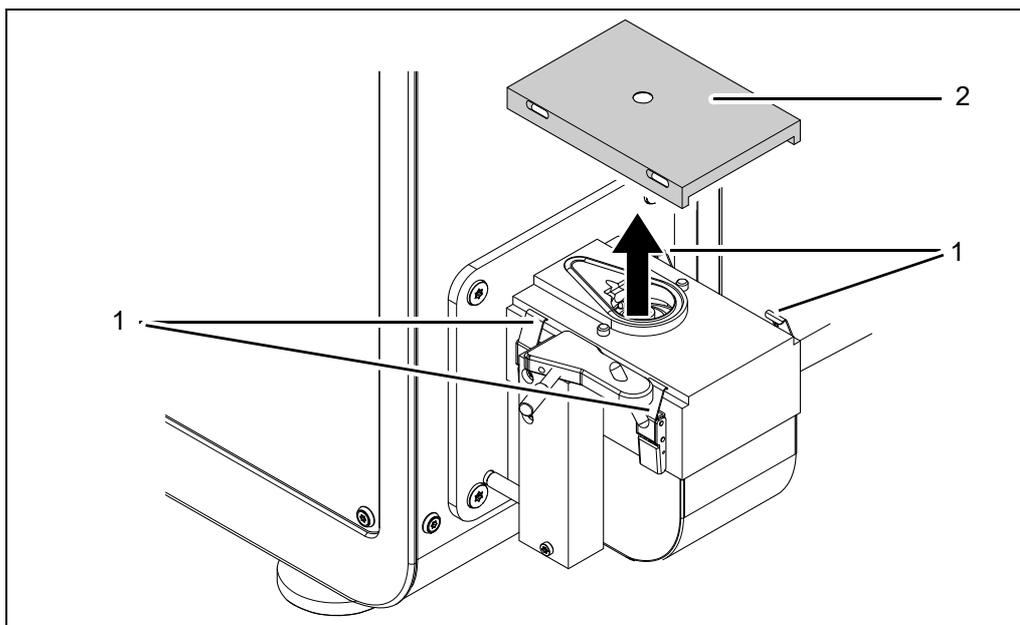
Fig. 9-2 Opening the spark stand plate
