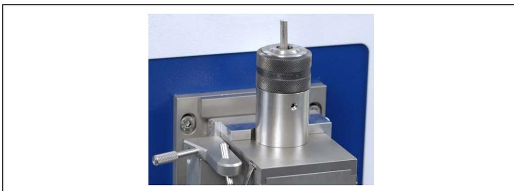
Fig. 9-12 "face-on" wire adapter on spark stand plate (example)
