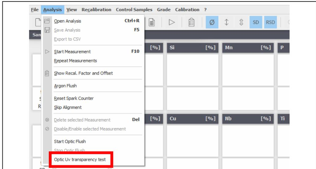
Fig. 5-8 Testing the UV transparency
