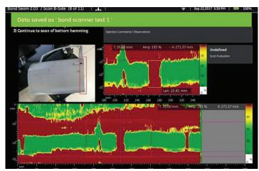
Green indicates strong adhesive bonding; Red indicates missing adhesive Note areas of slight adhesive leakage
