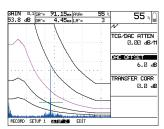
Tools for easy defect sizing Multiple curve DAC shows recorded DAC curve in magenta with 4 additional curves based upon dB Offset feature for added flaw sizing assistance. TCG Attenuation and Transfer Correction features make it very versatile for use on other materials and surface conditions.
